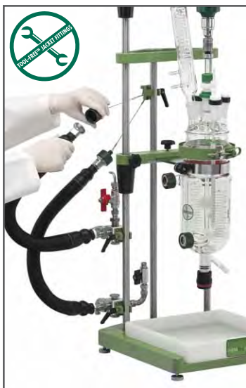
Tool-Free Jacket fittings with hose hanger incorporated into CHEMRxnHUB.
