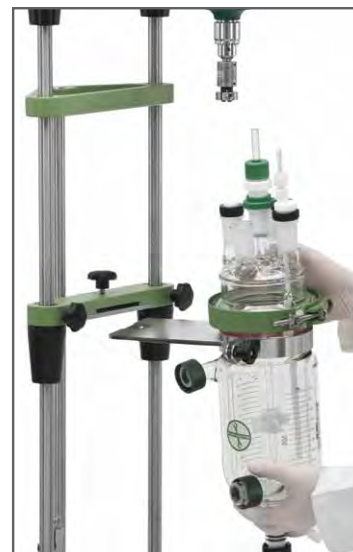
Unique clamp and support system provides simple installation and quick change-out.
